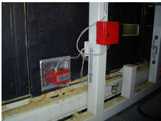
Illustration 4: Moisture measurement in the band weigher
