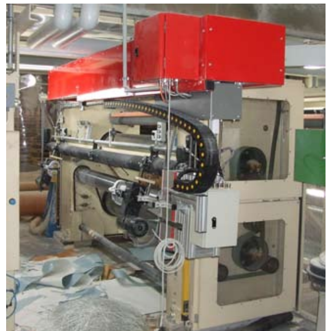
VenScan-LMS mounted behind the S-element (cooling roll)
